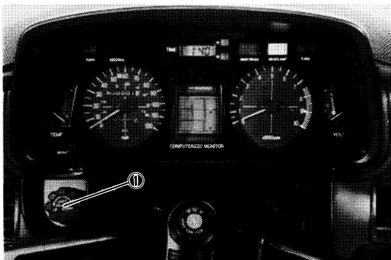
1. Headlight vertical adjusting knob
